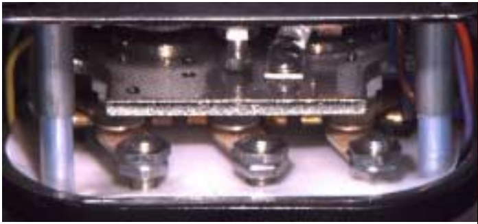
Figure 3 (above) – View of cut-open relay showing three contacts and sheet of Teflon insulation. Three (of six) contact pairs are visible directly below the armature. No evidence of contact arcing deposits can be seen.
